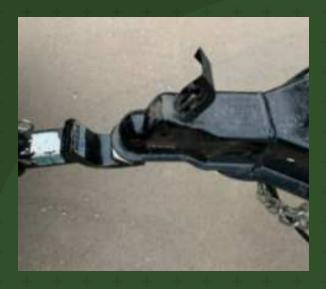
The hitch is a self-locking system. Pull it UP (like this) when installing it on the 2" ball. It will fully CLOSE & LOCK when dropped on the ball correctly.
