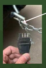
Ensure safety chains are connected to your vehicle's hitch brackets. There is extra chain length provided if you have a long hitch. This is for your safety, the teardrop, and, most importantly, others on the road.
